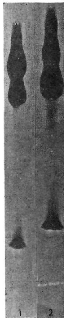
Fig. 2.—Chromatography of N'-substituted streptomycylamine preparations, period of development eighteen hours, mobile phase n -butanol-2% piperidine-2% p -toluenesulfonic acid: strip 1, N'- n -octylstreptomycylamine preparation; strip 2, N'- n -decylstreptomycylamine preparation.
